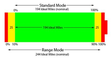
Many owners use only the default Standard mode and some don't fully understand Range mode, making collecting data on the full capacity of the battery pack challenging for those owners.
